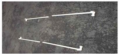
Once you are sure they are laid out and oriented correctly, one-by-one glue the corner assemblies to the rail pieces. When you are done, you should have 4 top rail pieces, each with one corner assembly permanently glued on the appropriate end as shown in the picture above.
